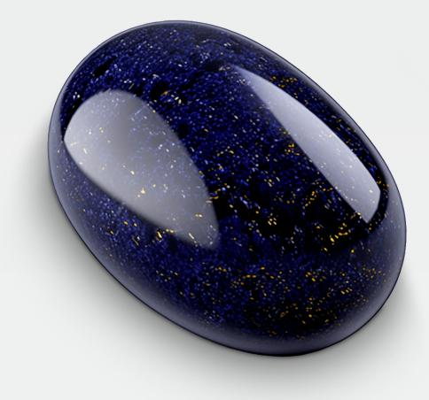
**Blue aventurine** is made of a coloring agent, silica, copper oxide and other metal oxide blended. Its flecked appearance and blue sparkling effect come from the combination, heated and cooled down process of the materials. Once the glass has sufficiently cooled and solidified, it can be shaped and polished to be placed within the dial. This full process ensures that each timepiece can be considered a unique work of art and engineering.
