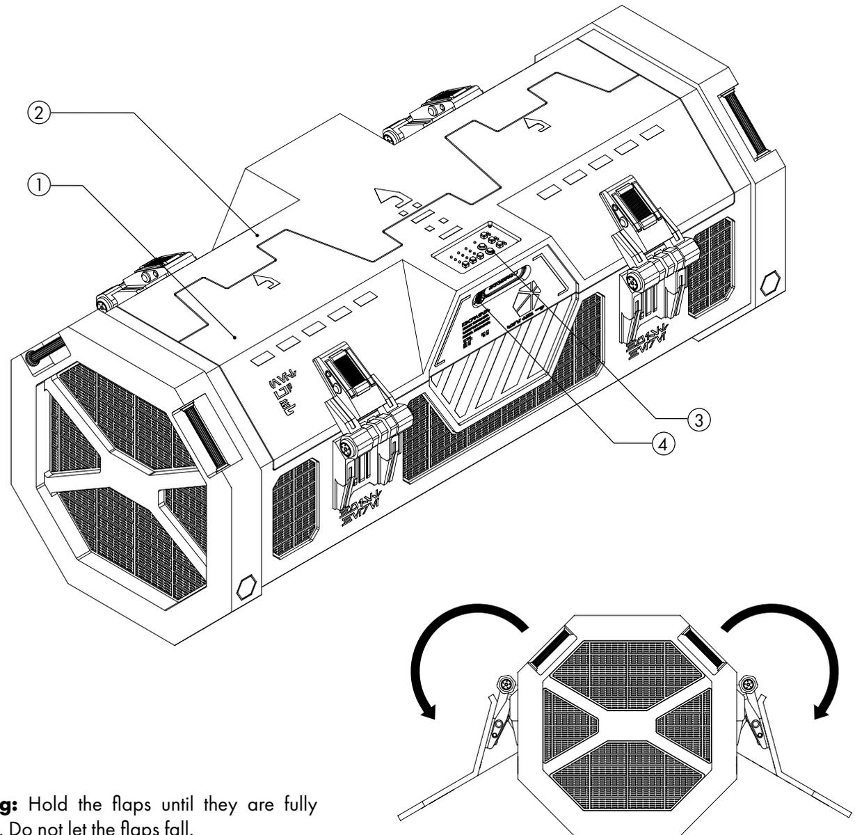
**Warning:** Hold the flaps until they are fully unfolded. Do not let the flaps fall.
